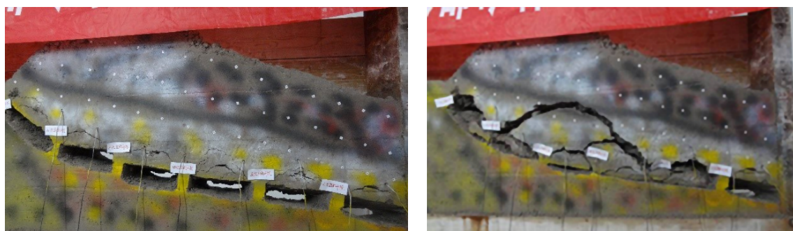
Fig. 2 Similar material simulation experiment of mining and pillar recovery.
