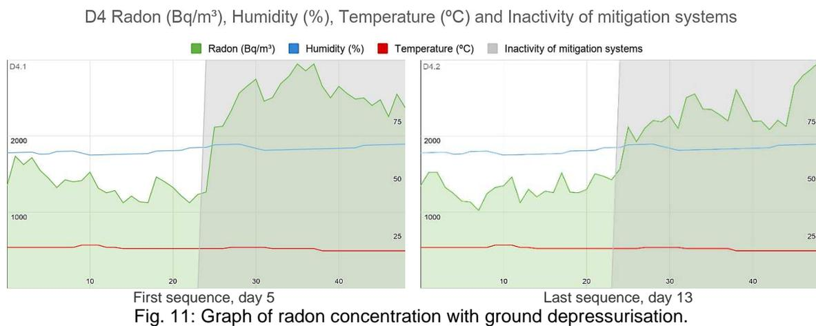
This solution proved not to be very effective in comparison with the previously tested solutions, although the limitations imposed on the method must be considered, since in order to minimize the degree of intervention it was decided to repurpose an existing manhole system.
