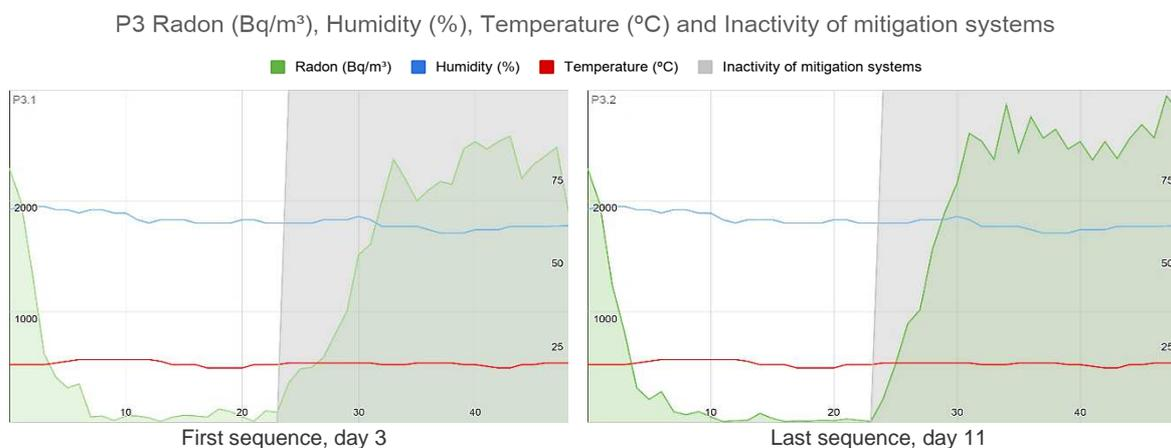
Fig. 9: Graph of radon concentration with the pressurisation system.
