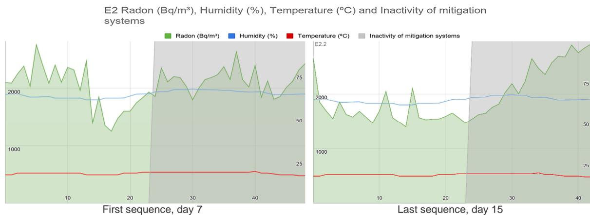
Fig. 13: Graph of radon concentration with the ground pressurisation.
