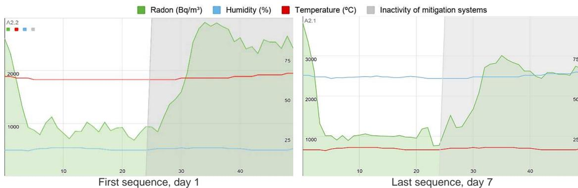
Fig. 7: Graph of radon concentration with the fan system operating.
