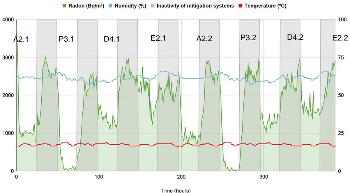
Fig. 14: Graph of radon concentration over the entire length of the experiment, showing the effect of sequential activating the various measures.
