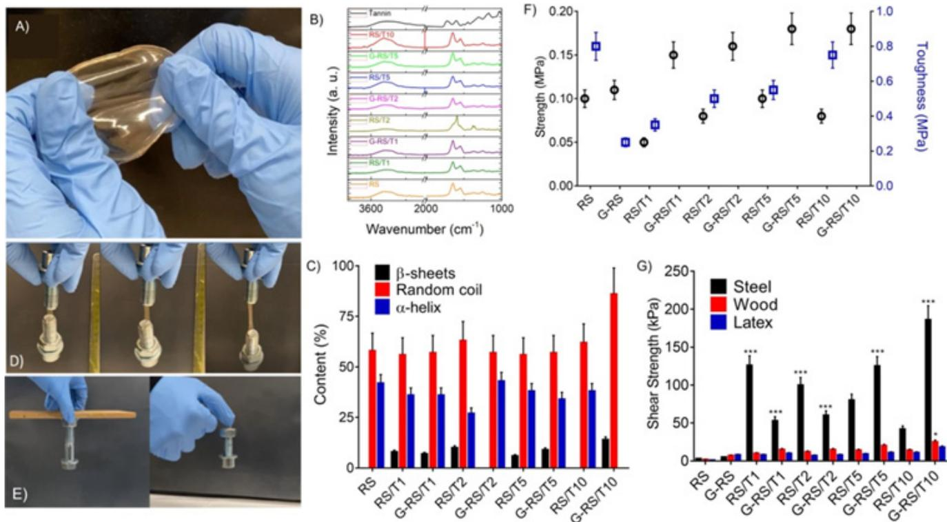
**Figure 3.** (A) Photograph of the RS/T10 composite. (B) FTIR spectra of neat RS, RS/T, and G-RS/T composites. (C) Structure composition of the prepared specimens. (D) Photographs showing the cohesive adhesion on stainless steel of the RS/T10 composite and tensile strength. (E) Adhesion of RS/T on wood (left) and latex (right). (F) The toughness of the prepared specimens was calculated from the engineering stress–strain curves. (G) Shear strength measurements of the ready models (13).
