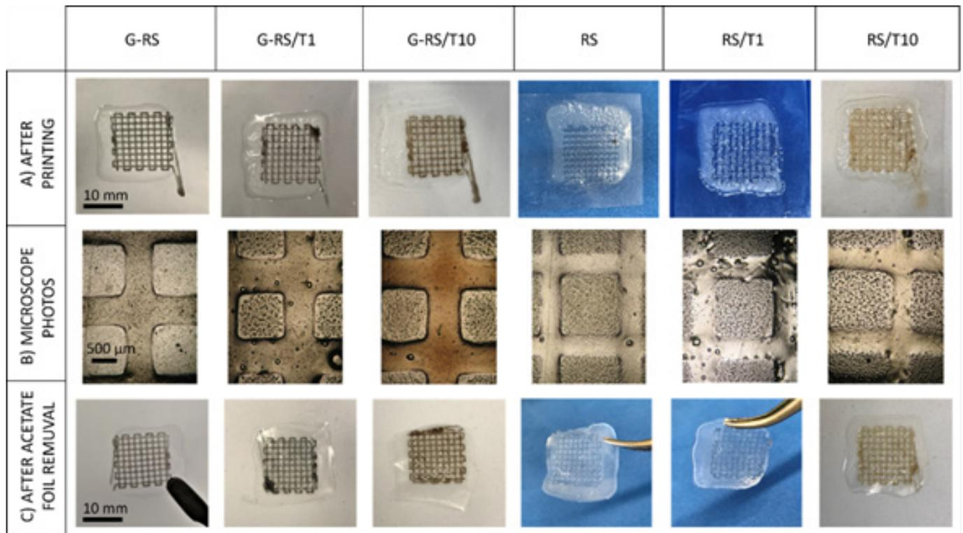
**Figure 2.** 3D printed grids based on RS, tannin, and GNP. A) Photos were taken as soon as the printing stopped. B) Photos obtained with a brightfield microscope. C) Photos of the structures after the acetate foil removal (13).
