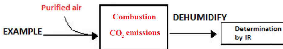
Fig. 3. Total organic carbon detection with Shimadzu SSM-5000A scheme
