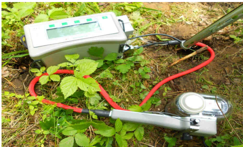
Fig. 4. ADC SRS-1000 for the measurements of CO 2 emissions from the soil
