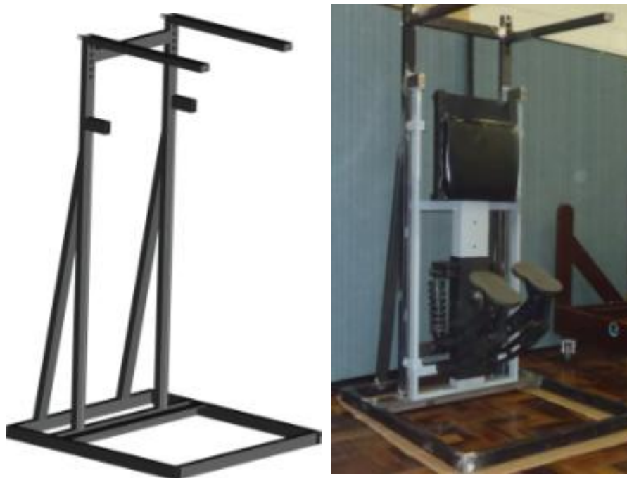
Figure 6. A 3-D CAD model, left, of the upright device that will support the multi-platform in a vertical position. The right photograph is the final integration of the multi-platform and the upright device.
