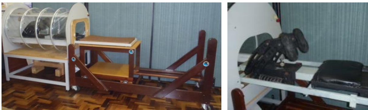
Figure 5. The left photo shows final integration of the multi-platform to the existing LBNP Box. The right photo displays a close up of the multi-platform outside of the LBNP Box.
