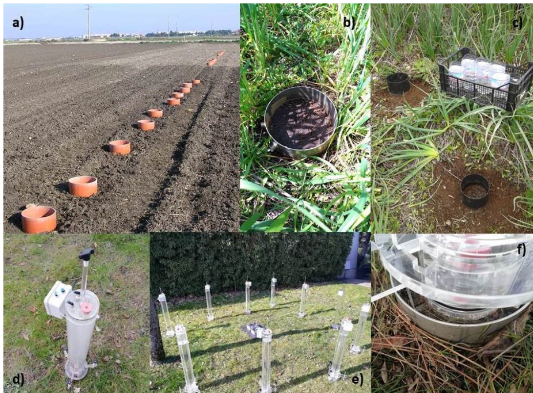
Fig. 5. Application of SFH (a) and BEST-Beerkan (b-e) methods in the field under different agro-environmental conditions, i.e., bare soil (a, d, e), winter wheat crop (b), Mediterranean maquis (c), and details of the automatic infiltrrometer (f).
