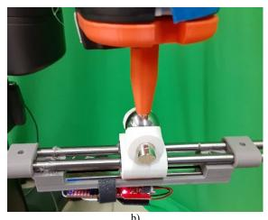
Fig.5. The fabricated Wireless Motion Gauge system: a) installed on two arms of a Baxter robot, b) the sensor module.
