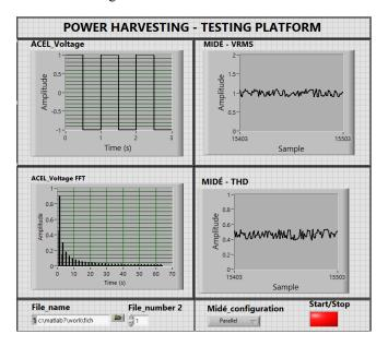
Fig.4. Front panel of the LabVIEW program used to display results of the acceleration data (left side) and power harvesting device (right side).
