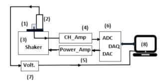
Fig.1. System block diagram: (1) accelerometer; (2) piezoelectric module; (3) vibration exciter; (4) charge amplifier (CH\_Amp); (5) power amplifier (Power\_Amp); (6) multifunction data acquisition board (DAQ); (7) voltmeter (Volt.); (8) laptop/smartphone.
