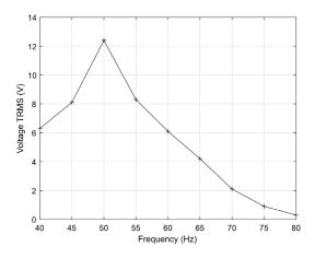
Fig.6. Frequency response of the power harvesting module tuned for a natural frequency of 50 Hz.
