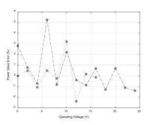
Fig.10. Relative error between experimental and polynomial curve fitted values.
