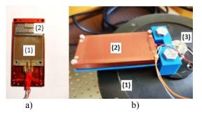
Fig.3. Piezoelectric module and vibration exciter used for testing purposes: a) Detailed view of the piezoelectric module and dimensional scale reference: (1) piezoelectric wafers; (2) tuning tip mass; (3) 1 € coin relative dimensional scale;
