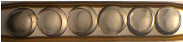
**Fig. 7.** Optical image of a  $^{125}\text{I}$  brachytherapy source consisted of six  $^{125}\text{I}$  seeds within a glass tubing. The overall diameter of the seeds was  $600\ \mu\text{m}$ , and the diameter of core was  $500\ \mu\text{m}$ .
